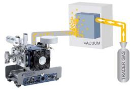
Fuel cell bipolar plates are typically tested in a vacuum chamber leak test due to low leak rate requirements and need for high throughput.
